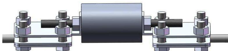
provides an insulating gap between the installation and the earth. There occurs a short-circuiting inside the magneto in the case of a lightning discharge, which ensures the flow of the electric current of the thunderbolt to the earth. Among other applications, it is used for the protection of antenna masts.
